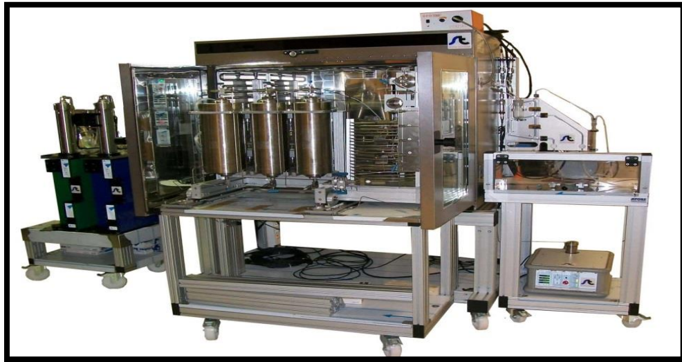
Figure 2.29: Slim-tube experiment setup
